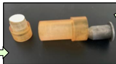
Centrifuge insert assembled with filter & cone
