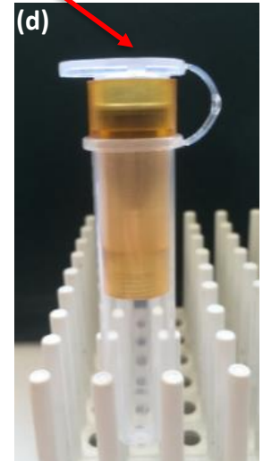
Centrifuge tube cap presses cone into filter
