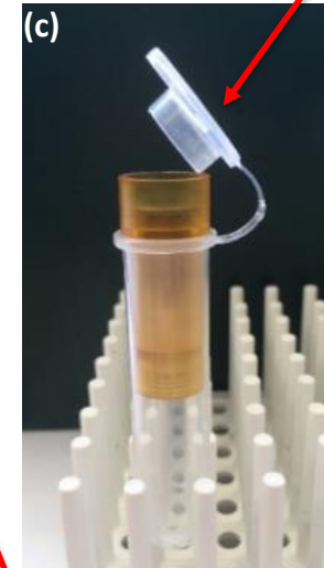
Centrifuge tube cap presses cone into filter
