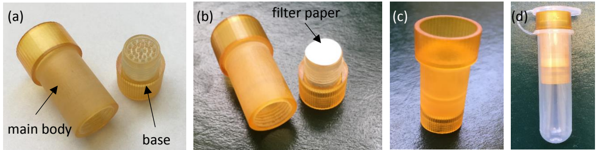
Figure 3.4: 3-D printed insert. (a) Main body and base of insert. (b) Filter paper sitting on top of the base. (c) The base screwed into the bottom of the main body. (d) The insert sitting inside a centrifuge tube.
