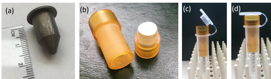
Figure 5.1: (a) Metal cone. (b) Insert with filter paper placed on the base. (c) Metal cone inside the insert which is inside a centrifuge tube. (d) Cap of centrifuge tube presses metal cone into filter paper sitting on the base of the insert.
