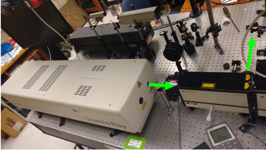
Figure 2.3: Picture of 355 nm Nd:YAG with arrows representative of laser light pumping the OPO, resulting in a signal beam, shown reflecting out of the OPO orthogonally.
