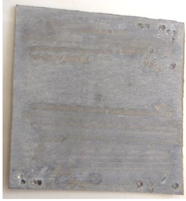
Figure 4.3: A camera picture of the neodymium platelet used as the target for both single and dual pulse LIBS experiments.
