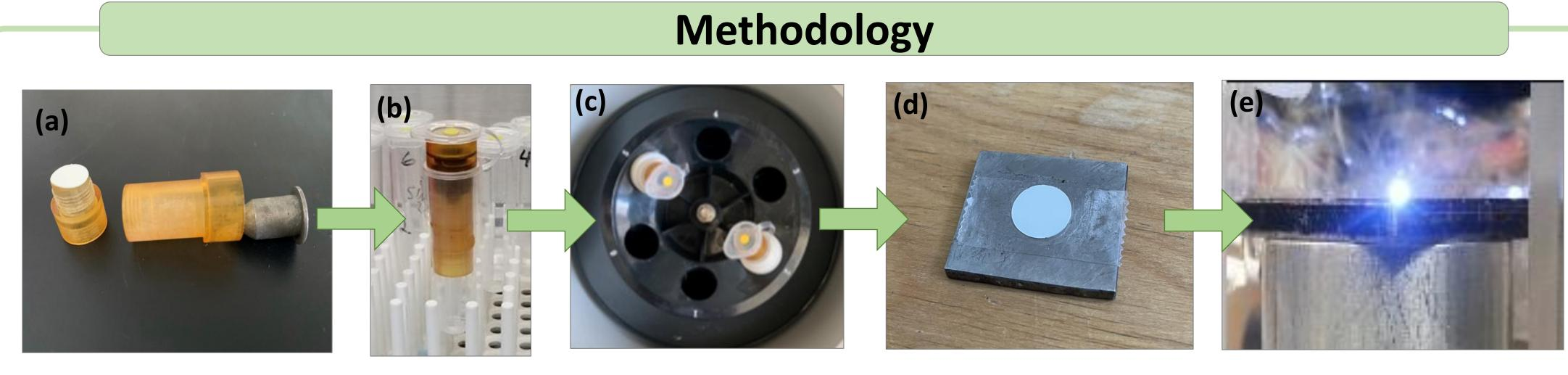
(a) A 3D-printed centrifuge insert which has a metal cone attachment is assembled and placed in a test tube (b) where bacteria is concentrated onto a nitrocellulose filter. (c) The sample is centrifuged and then the filter is mounted onto a piece of steel (d) which is then placed in an argon environment and ablated by a 1064 nm ND:YAG laser (e). Finally, a broadband atomic spectrum is obtained.
