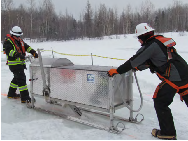
At left, an ice cutter chainsaw sled creating a space for oil to collect. At right, oil between the water and ice collects in the trench for easier clean-up. Source: ECRC, Cold Weather Training Document, provided to authors, 2023.
